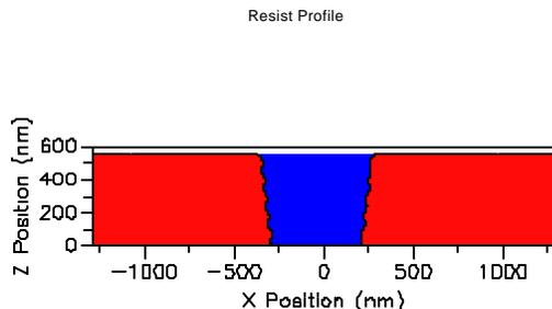
Figure 15: IP3600 resist profile with an organic ARC
