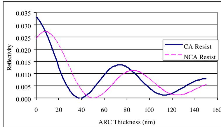
Figure 5: Simulation of the optimal ARC thickness to minimize reflectivity for a NCA and CA resist at 257 nm
