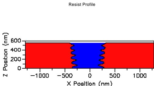
Figure 14: IP3600 resist profile without an organic ARC
