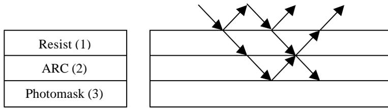
Figure 1: Optical Film Stack with the use of an Antireflection Coating
