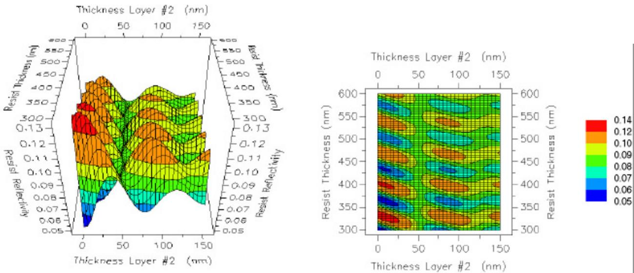
Figure 18: Resist reflectivity as a function of ARC and photoresist thickness for a 257 nm NCA resist process
