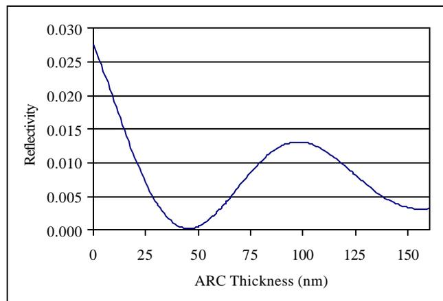
Figure 3: Simulation of the optimal ARC thickness to minimize reflectivity for IP3600 at 365 nm
