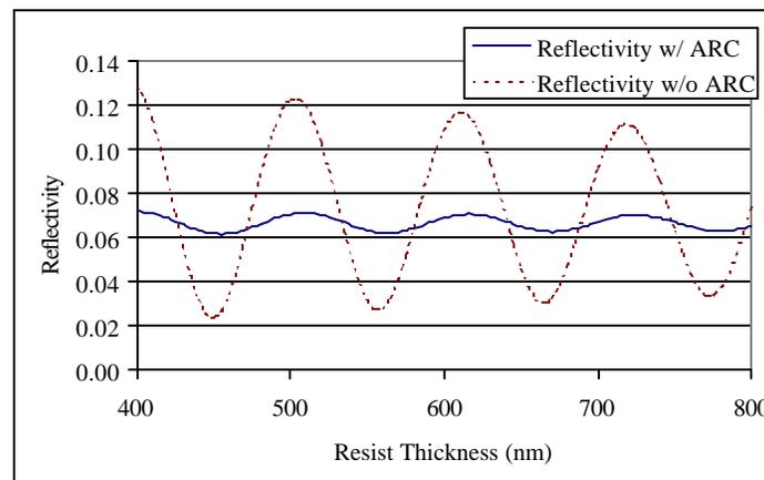
Figure 4: Simulation of the swing ratio reduction for IP3600 using the optimal Organic ARC thickness for 365 nm
