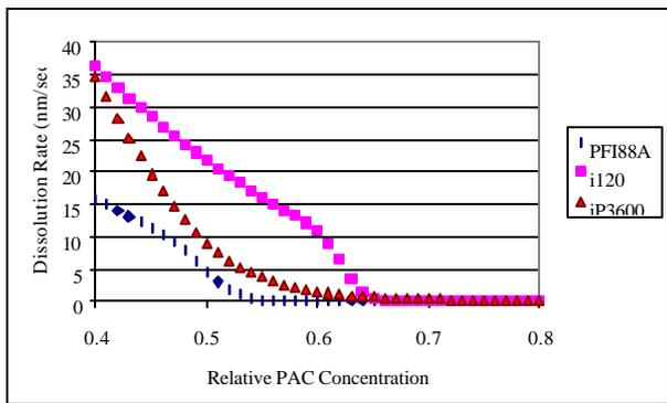
Figure 13: Dissolution Rate model for three I-line photoresists
