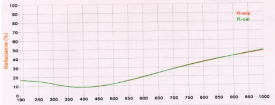
Figure 2: Reflectivity on Hoya AR3 photomask coatings as a function of wavelength
