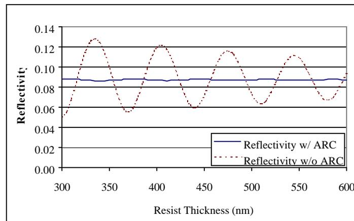
Figure 6: Simulation of the a NCA resist with and without an organic ARC at 257nm
